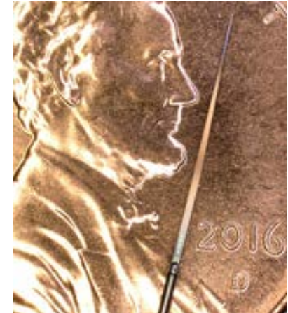
Left: 16- and 32- channel Vector Arrays Below: 64-channel Vector Array on a US penny
