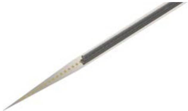
Illustration showing flat optical fiber mounted on an electrode array shank.
