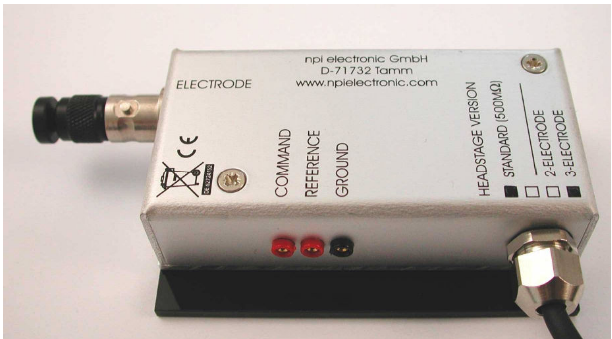
Figure 4: VA-10X 3 electrode headstage with CFE electrode holder (optional)
