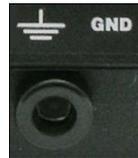
The **VCPLUS** controller can be connected to ground via a 4mm banana jack on the rear panel.
