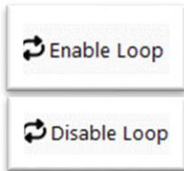
This button will enable or disable a loop created in a sequence. Only one loop can be created in a sequence. A loop will not be saved, so it is best to note where the loop is in case you need to add it again.
