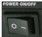
The **VCPLUS** valve controller has two power switches. The main power is located on the rear of the unit. This rocker switch will turn input power ON or OFF to the system.
