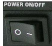
Power ON/OFF switch will turn the main power to the controller ON or OFF.
