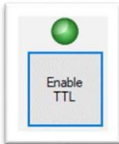
Enables/disables the trigger in function. The trigger function is utilized via the 8 pin Digital In on the back of the **VCPLUS** controller. You must input a trigger at the pin corresponding to the valve selected in the row. Check the box “Wait for Trigger” and the program will pause until a TTL is sensed at the pin corresponding to the valve number. Then the sequence will continue. ALA BOB-8 breakout box can be used.
