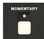
To enable the membrane switches to act as momentary switches press the “MOMENTARY” button on the controller. A green LED will indicate the momentary setting is enabled. In the momentary mode you must press and hold down the membrane switch to energize, turn ON, a valve. As long as you hold down the switch the valve remains ON. Release the switch and the valve turns OFF.
