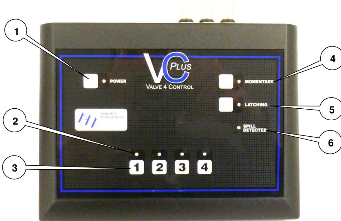
1. **Soft Power Button with LED** - Green LED indicates when system is powered. It is also used to reset the spill sensor alarm.
