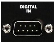
The digital input is used to control the valves via a TTL signal. The DB-9 male connector pins 1-4 is used to input TTL signals to valves 1-4, respectively, with pin 9 being common ground.
