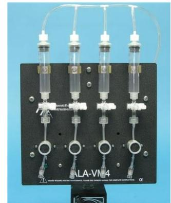
Since there are several possible front-end manifolds and tubing choices, both the **VCPLUS4-PP** and the **VCPLUS4-CLP** systems are sold configured up to the valve inputs. This allows the user to connect the valve outputs to their choice of front-end tubing and manifold. The user also has the option to include one of our focal perfusion manifolds and accessories in their order (see the options section).
