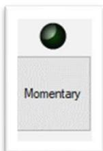
This button will switch the valve buttons from being toggled to momentary. When the button is gray, the toggle mode is enabled. When green, the valve stays ON while the mouse button is held down over its valve button, release the mouse button and the valve turns off.
