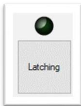
Enables/disables the latching mode of the **VCPLUS** controller. The button will go green when enabled. The Latching lamp on the controller will also turn ON. When enabled the valve that is switched ON will be switched OFF when any other valve is switched ON. Only one valve can be ON at a time in this mode. This feature allows for fast manual solution switching by eliminating the need to switch a valve OFF before switching another ON.
