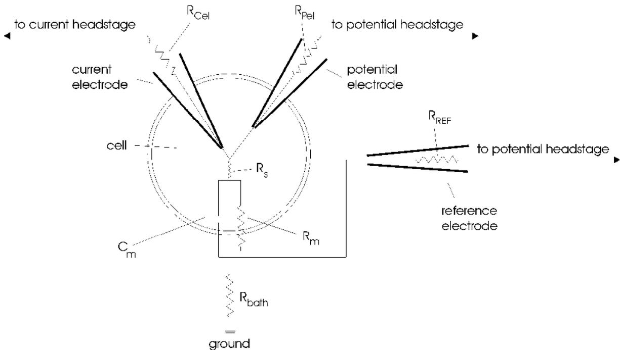
Figure 15: model circuit for voltage clamp recording from a cell, e.g. an oocyte using low-resistance electrodes
