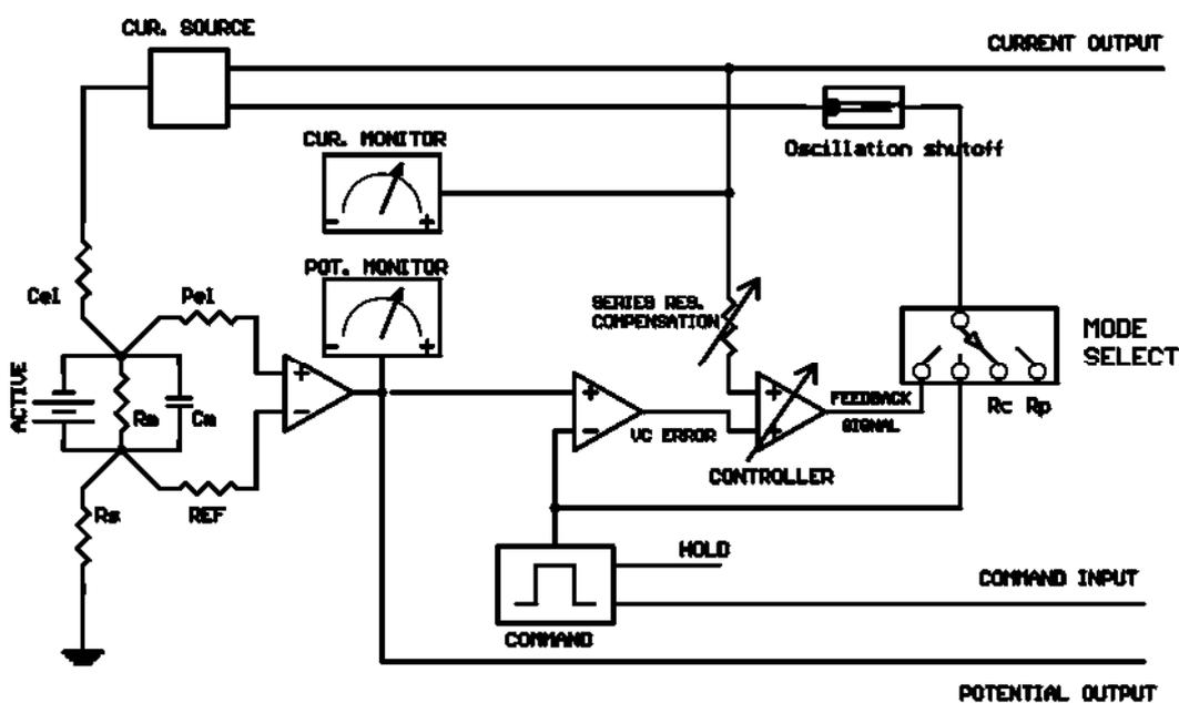
Figure 1: equivalent circuit of TEC amplifiers
