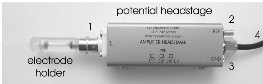
Figure 6: potential headstage and electrode holder (optional)
