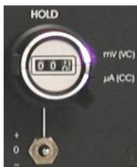
The HOLD unit consists of (12) HOLD current / potential potentiometer and (25) + / 0 / - switch.
