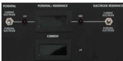
The DISPLAY unit consists of (7) electrode selector for POTENTIAL, (8) mV LED, (9) CURRENT display, (10) POTENTIAL / RESISTANCE display, (11) MΩ LED and (13) electrode selector for RESISTANCE.
