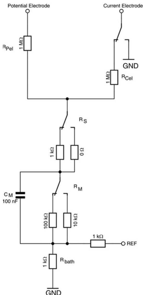
Figure 11: schematic diagram of the TEC passive cell model
