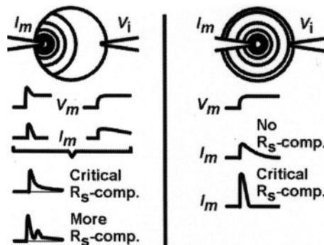
Figure 13: penetration depth of the current electrode and consequences for the clamp
