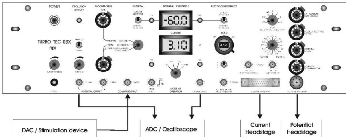
Figure 9: basic electrical connections
