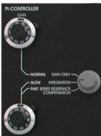
The voltage clamp control unit consists of **(5)** GAIN potentiometer, **(4)** PI-CONTROLLER potentiometer and **(6)** control mode switch (see also chapter 8.6).
