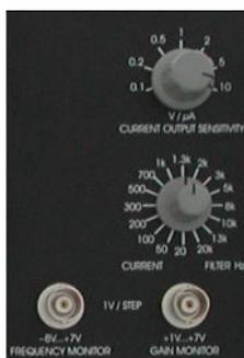
The CURRENT OUTPUT conditioning unit consists of (14) CURRENT FILTER Hz, (15) V /  $\mu$ A CURRENT OUTPUT SENSITIVITY, (21) +1V...+7V CURRENT OUTPUT SENSITIVITY MONITOR connector and (23) -1V...+7V FREQUENCY MONITOR connector.
