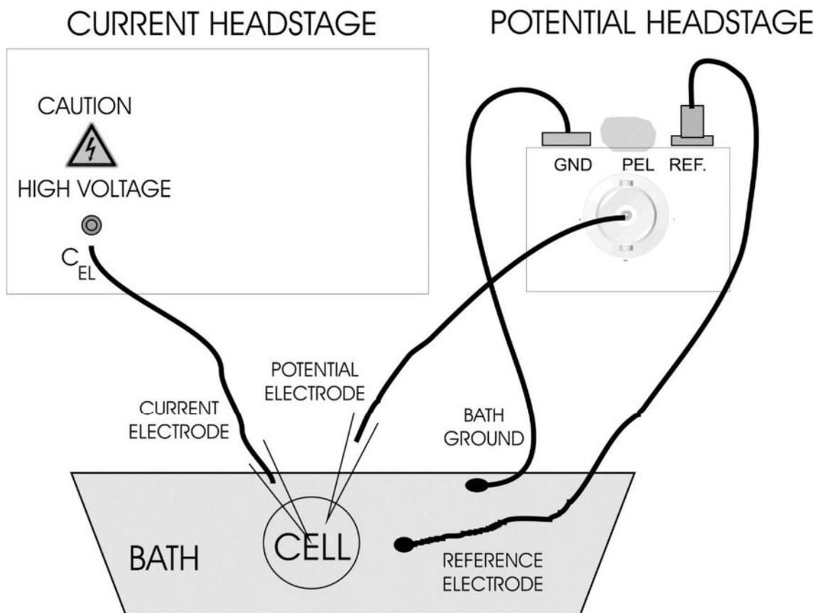
Figure 8: connections of the headstages
