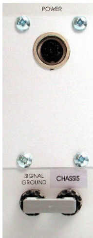
Figure 4: Rear panel connectors of the EPMS-E-07
