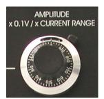
Ten-turn potentiometer for setting the AMPLITUDE of the output signal. Range in VOLTAGE mode: 0.1-99.9 V. Amplitude in CURRENT mode is the reading of this potentiometer multiplied by the factor set with switch #20.
