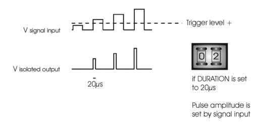
Direct mode (input at SIGNAL INPUT BNC)
