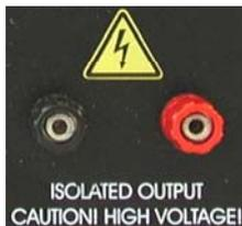
Jacks providing the ISOLATED OUTPUT signal. The polarity of the input of the +,0,- switch (#19, Figure 5) respectively is not changed, i.e. the red plug is positive (+) if the output polarity switch is set to + or the input signal is positive. This signal is completely isolated from earth. The black jack serves as reference point for the isolated output signal. The black banana connector of the supplied cable is connected to the black jack and the red to the red jack.
