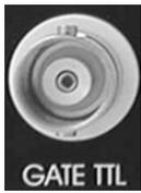
BNC connector for triggering the stimulus isolator in GATE TTL INPUT MODE (see also chapter 5).
