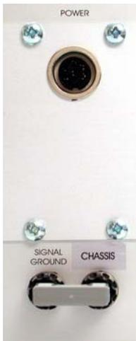
The 19" cabinet is connected to the CHASSIS connector at the rear panel. It can be connected to the SYSTEM GROUND (SIGNAL GROUND) on the rear panel of the instrument (see Figure 4).
