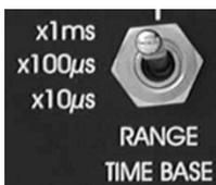
Three position switch to set the time base of the built-in timing unit. Available ranges: 10-99  $\mu$ s (lower position), 100-999  $\mu$ s (middle position), 1-99 ms (upper position).
