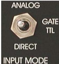
Three position switch to set the operating mode of the stimulus isolator either to ANALOG, to GATE TTL or to DIRECT INPUT MODE (see also chapter 5).
