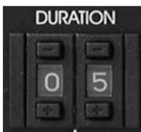
2-digits, digital potentiometer to set the stimulus duration in GATE TTL INPUT MODE. The stimulus duration is the reading of this potentiometer multiplied by the factor set with switch #16.
