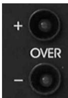
LEDs indicating when the isolator exceeds it's linear range limit ( $\pm 90$  V or  $\pm 9$  mA respectively).
