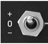
Switch for setting the polarity of the output signal in GATE TTL INPUT MODE. In “0” position the internal stimulus generation is disabled
