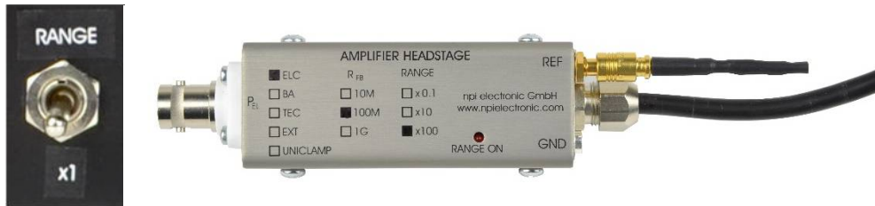
Figure 8: Current RANGE switch (left) and ELC switchable headstage (right).
