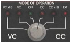
Switch for selecting the MODE OF OPERATION
