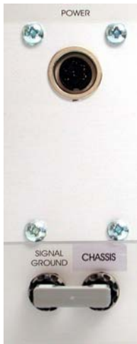
Figure 4: Rear panel connectors of the EPMS-E-07
