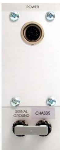
Figure 4: Rear panel connectors of the EPMS-E-07
