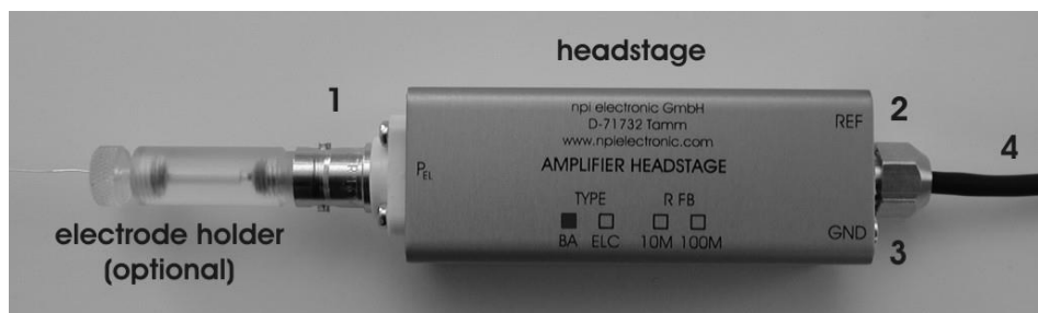
Figure 6: electrode holder (optional) and headstage of the BA-03X
