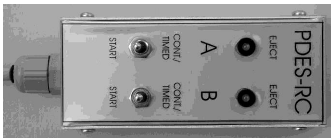
Figure 6: PDES remote control (optional)
