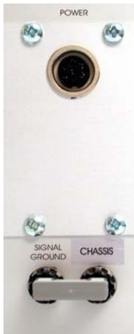
Figure 4: Rear panel connectors of the EPMS-E-07
