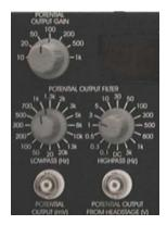
The POTENTIAL OUTPUT unit consists of (2) POTENTIAL OUTPUT GAIN, (34) POTENTIAL OUTPUT FILTER HIGHPASS (Hz), (35) POTENTIAL OUTPUT FROM HEADSTAGE (V), (36) POTENTIAL OUTPUT (mV) and (37) POTENTIAL OUTPUT FILTER LOWPASS (Hz).
