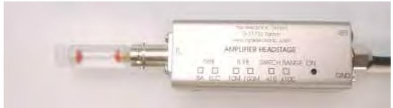
Headstages with switchable feedback resistor (x1/x10 or x1/x100) allow higher effective voltages for electroporation, or (x1/x0.1) better current resolution for patch-clamp experiments
