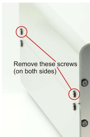
Figure 4: Lid screws to be removed to open the FiberOptoMeter-III housing.
