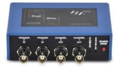
Output: 11 bits resolution +/- 5 V DC to 50 kHz (single channel 100 kHz)
