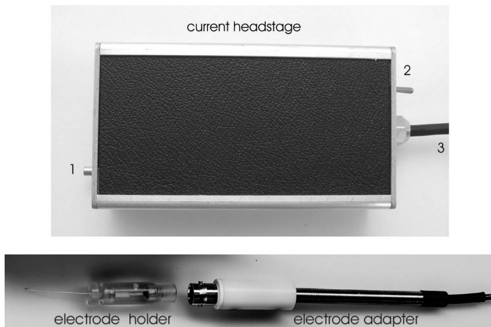
Figure 7: current headstage with (optional) electrode holder and (optional) electrode holder adapter of the TEC-03X system
