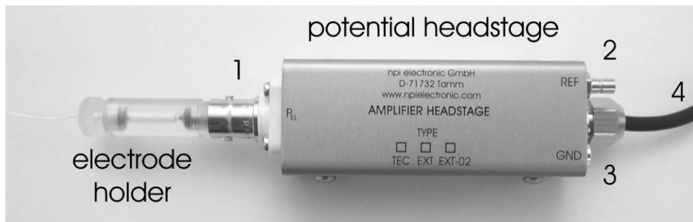
Figure 6: potential headstage and electrode holder (optional)
