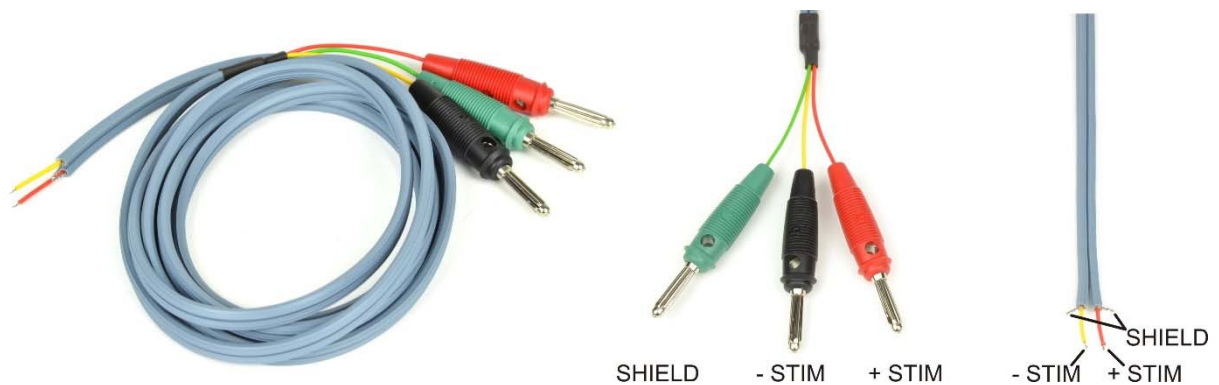
Figure 2: ISO-CAB - shielded cable for connection of stimulation electrodes.
