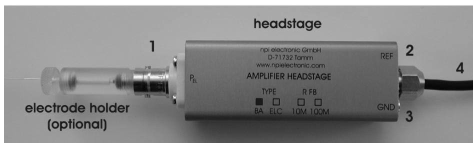
Figure 6: electrode holder (optional) and headstage of the BA-01X
