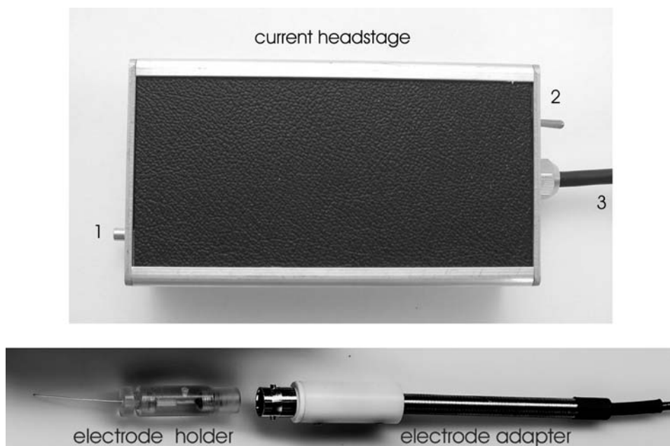
Figure 9: current headstage with (optional) electrode holder and (optional) electrode holder adapter of the TEC-03X system
