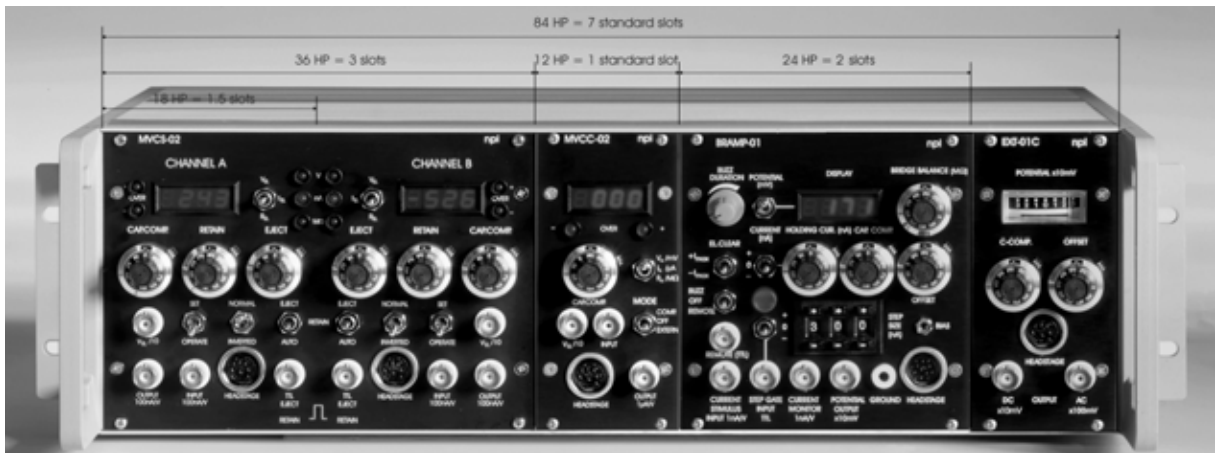
Figure 1: Example of a measurement system located in an EPMS housing with two channel iontophoresis and balance module (MVCS-02, MVCC-02), bridge amplifier module (BRAMP-01R) and an extracellular amplifier module (EXT-01C)
