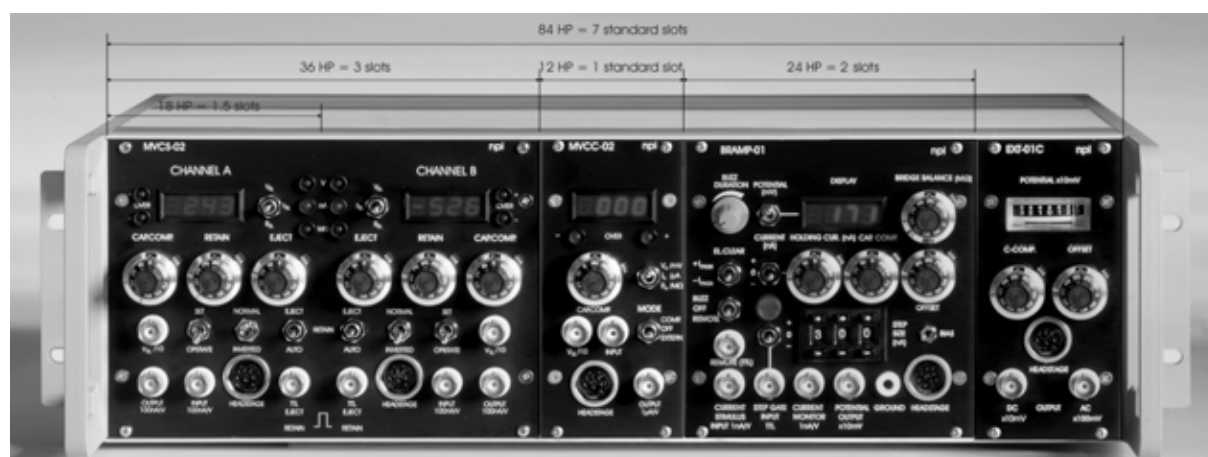
Figure 1: Example of a measurement system located in an EPMS housing with two channel iontophoresis and balance module (MVCS-02, MVCC-02), bridge amplifier module (BRAMP-01R) and an extracellular amplifier module (EXT-01C)
