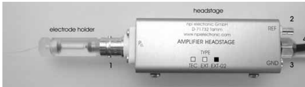
Figure 3: headstage (optional) and electrode holder (optional) and of the EXT-02F
