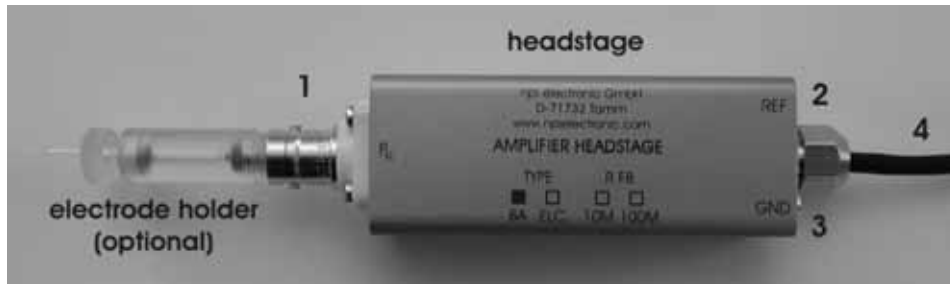
Figure 6: electrode holder (optional) and headstage of the BRAMP-01R
